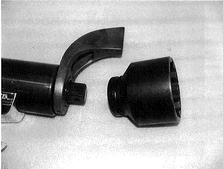
Figure 6. Installing jGun Socket
