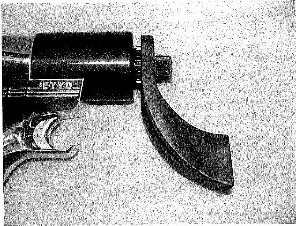
Figure 4. Reaction Arm Installed
